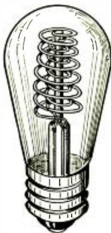
Fig. 2—German type of neon scanning tube, containing two wire spirals inside the bulb, the space between them becoming filled with a luminous glow. A lens in front of the tube gives the same optical effect as a flat plate.
