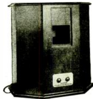
An early American television unit incorporating scanning disk, neon lamp, television frequency amplifier and power supply.
