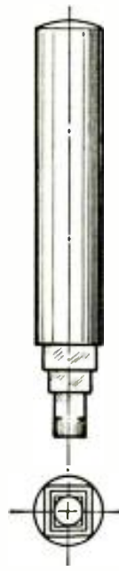
Fig. 4. Punch for square holes, with other punches each slightly larger (purposely exaggerated in the figure).
