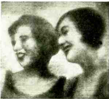
Appearance of image reproduced on the end of Von Ardenne's cathode ray tube (un-retouched photo).
