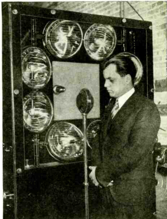
Mr. Sanabria is here seen standing in front of his television transmitter—note the bank of photoelectric cells which pick up reflected light rays falling on his face when being scanned.
