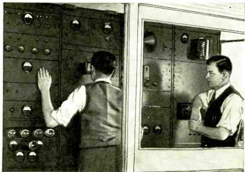
Here we have the control board of W2XCR, located two floors above the 5 k.w. "power transmitter" shown above. The television image is also monitored at this board.
